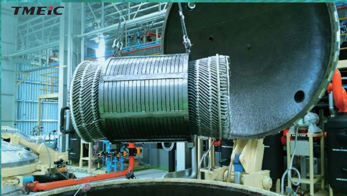
Installing stator in VPI tank
