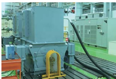
Combined test with inverter drive
